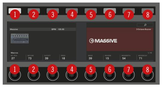
The unlabeled buttons and knobs on the KOMPLETE KONTROL S-Series keyboard.
