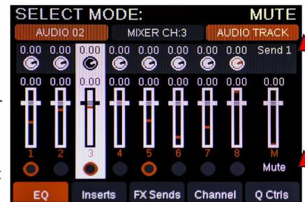
The 8 LED buttons below the faders are by default assigned to Select. Try pressing first LED button 1 and then LED button 8. Notice this is a quick way to jump from one track to another.
