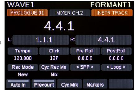
Below the SPP readout you see the position of the Left and Right locators (or start time and end time of time selection). You can set the locators to the current song position by pressing [Shift]+[Goto L] and [Shift]+[Goto R]
